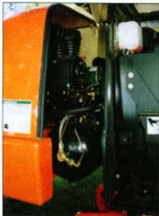
The SkyAir compressor securely fits behind the boom lift's engine, hidden from all except for the pressure gauge mounted in the platform.
